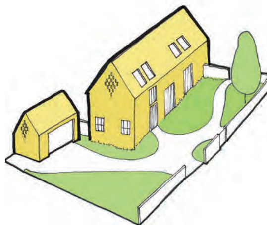
This barn conversion retains the original building outline using flush fitting conservation roof lights. The original barn openings have been retained, and therefore the windows and doors retain their original proportions as much as possible. The new windows have been created in the less visible end gable by opening (but not enlarging) the blocked window and creating a new window alongside. The ventilation holes have been retained with internal glazing.
